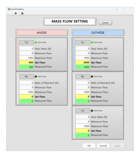
The settings can be adjusted in two modes: 'Normal' and 'Load Follow'. You can switch between these modes by clicking the [Normal] button at the top to switch to [Load Follow].
