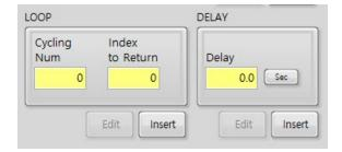
The LOOP feature in the Test Sequence is used to repeat a specific section of the sequence. When the Test Sequence reaches a LOOP item, it returns to the line specified in "Index to Return" and repeats this process for the number of times indicated in "Cycling Num". For example, if the LOOP item is on line 6 with a Cycling Num of 2, and Index to Return is 3, the sequence will operate as follows:
