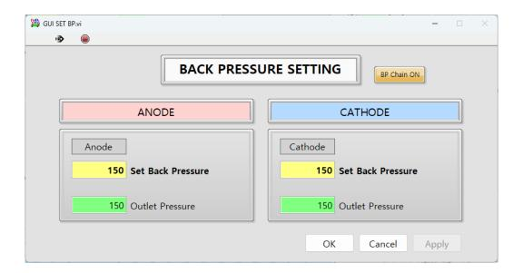
If pressurization is necessary, you can set the pressure for the Anode and Cathode lines. The 'BP Chain' mode can be turned on or off using the button at the top.
