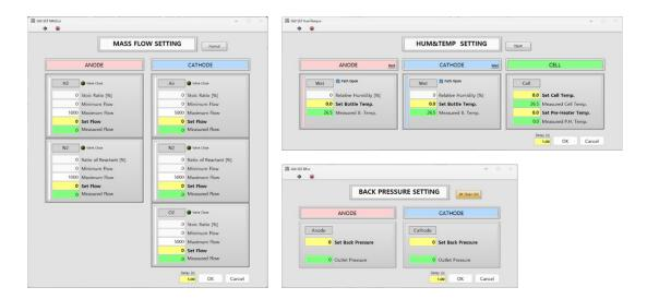
The [MASS], [HUMI&TEMP], and [Back Pressure] buttons at the top of the central section open a settings window similar to the Manual Control described in Chapter 3. The usage is the same as previously explained. However, there is an option at the bottom to enter a Delay, which represents the time delay between the execution of a setting and the next one. The [OK] button can be used to insert these settings into the Test Sequence.
