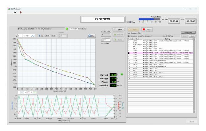
The image shows the state while the protocol is in progress. When the protocol is running, the data saving path of the protocol is displayed in the upper left corner of the screen. Right below it is the I-V Curve chart, which draws a trajectory as the I-V Trip of the electrical load progresses. Additionally, there is a chart below that allows real-time monitoring of data measured from the electrical load.
