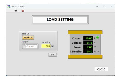
Here, you can remotely set the electrical load. After selecting the Load On/Off status, the target mode (Current, Voltage, Power), and entering the value, clicking the [Set] button activates the electric load.
