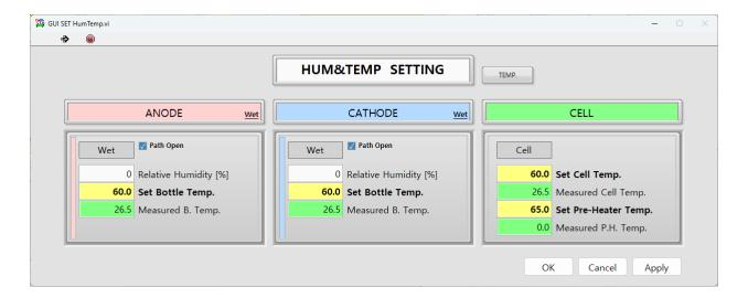
The humidification of gases for the Anode and Cathode can be set in either Temperature Mode or Relative Humidity Mode. To switch modes, click the [TEMP.] button at the top to toggle to [R.H].
