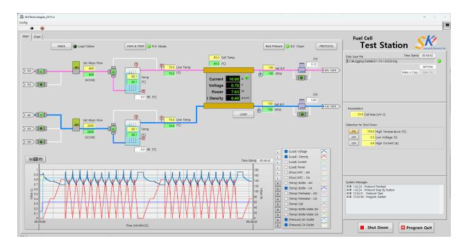
At the bottom right of the Main panel, there is a [Shut Down] button to reset the components of the test station to their initial state, and a [Program Quit] button to exit the program. The [Program Quit] button is programmed to perform a shut down before exiting the program, but for safety, it is strongly recommended to manually proceed with [Shut Down], verify the status of the test station, and then exit the program.
