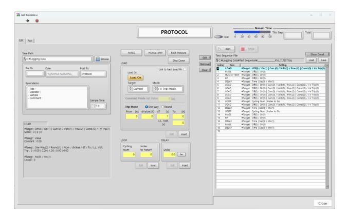
In the protocol, you can write and execute test sequences according to user needs, utilizing gas flow, temperature and humidity, back pressure, and load operations for automatic execution. In the top left section, there's a setting area for the file where protocol results are saved. In the right section, you can review the written test sequences. The central section contains buttons and boxes for entering commands that go into the test sequences.
